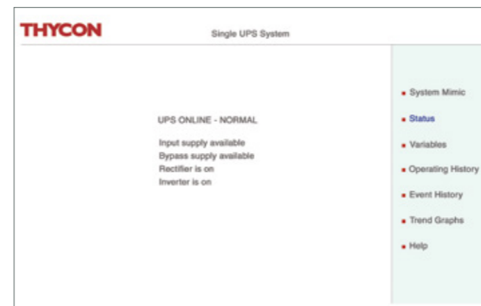
UPS power system monitor - status
