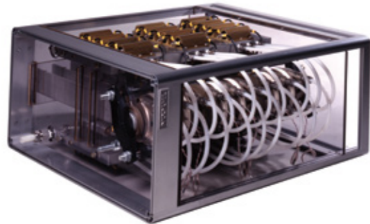
3 phase 5MVA thyristor converter
