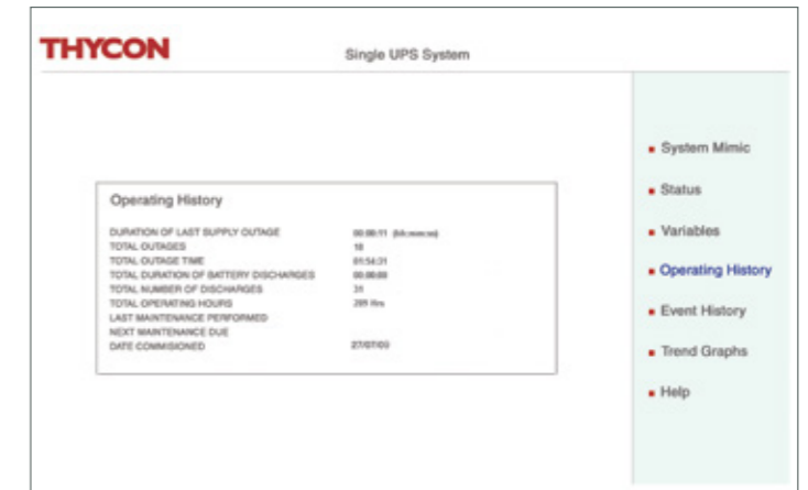
UPS power system monitor - operating history
