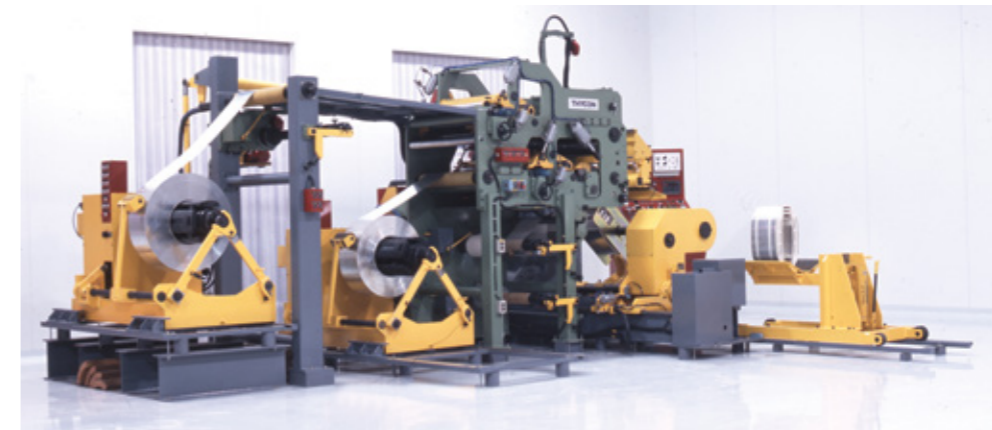
Bifilar transformer foil and strip winding machine
