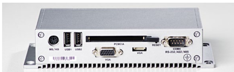
Thycon power system monitor (front)
