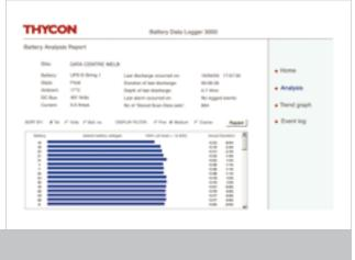
The BDL does not require any proprietary software. Simple to use and flexible, it provides unsurpassed monitoring capabilities to achieve peak battery performance and long service life. The BDL sorts battery voltage deviations into five user-definable tolerance bands (typically 2%, 5%, 8%, 10% and 20%). Requests for data are read in real time, analysed and then presented to the user.
